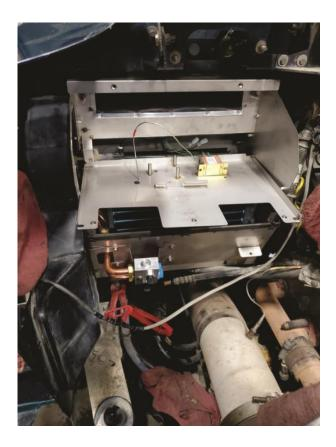
8. Install the blower motor. Connect the blower motor wiring and reattach the blower motor to the baffle plate.
