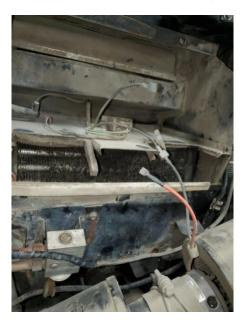
4. Remove the pair of 8mm nuts from the freeze switch.
