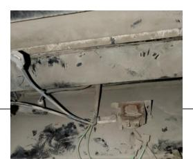
5. Unscrew the three Philips screws from the recirculation door actuator. (Note: This step might slightly differ if your truck uses an air-operated actuator.)
