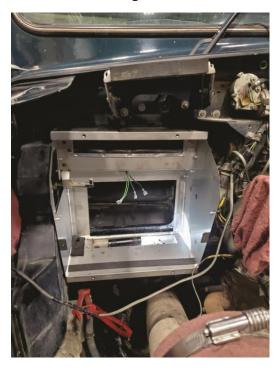
2. Secure the heater box using the provided nuts and bolts. Insert the top two bolts through the recirculation door flap. Use a wrench on the bolt side and tighten the nuts with a ratchet.
