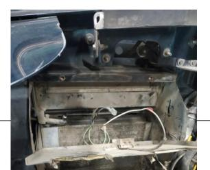
7. Detach the two coolant lines that connect to the heater core. Use hose clamps or hose clamp pliers to avoid coolant loss.
