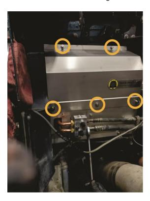
10. Re-attach hoses and any other original accessories to your new stainless steel Kenworth heater box from truckpartsline.com.
